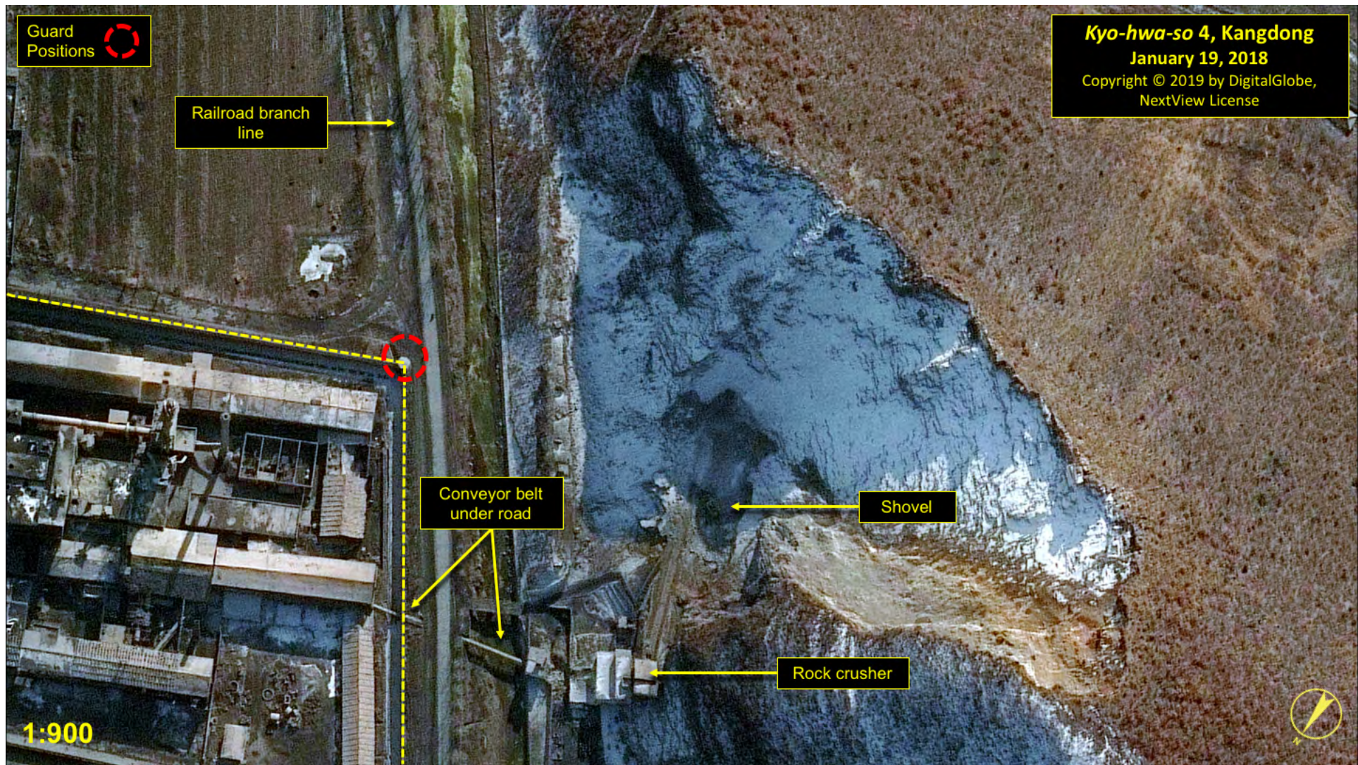
A close-up of the limestone quarry adjacent to Kyo-hwa-so No. 4 on January 19, 2018.
