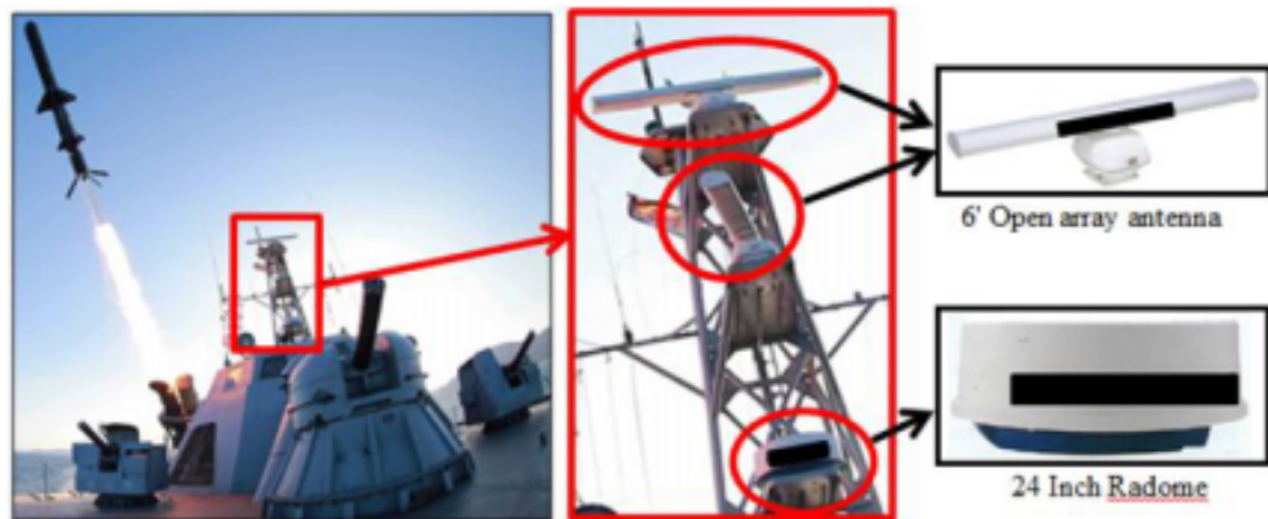
Figure 24 Commercial radar antennas adapted for naval vessel
